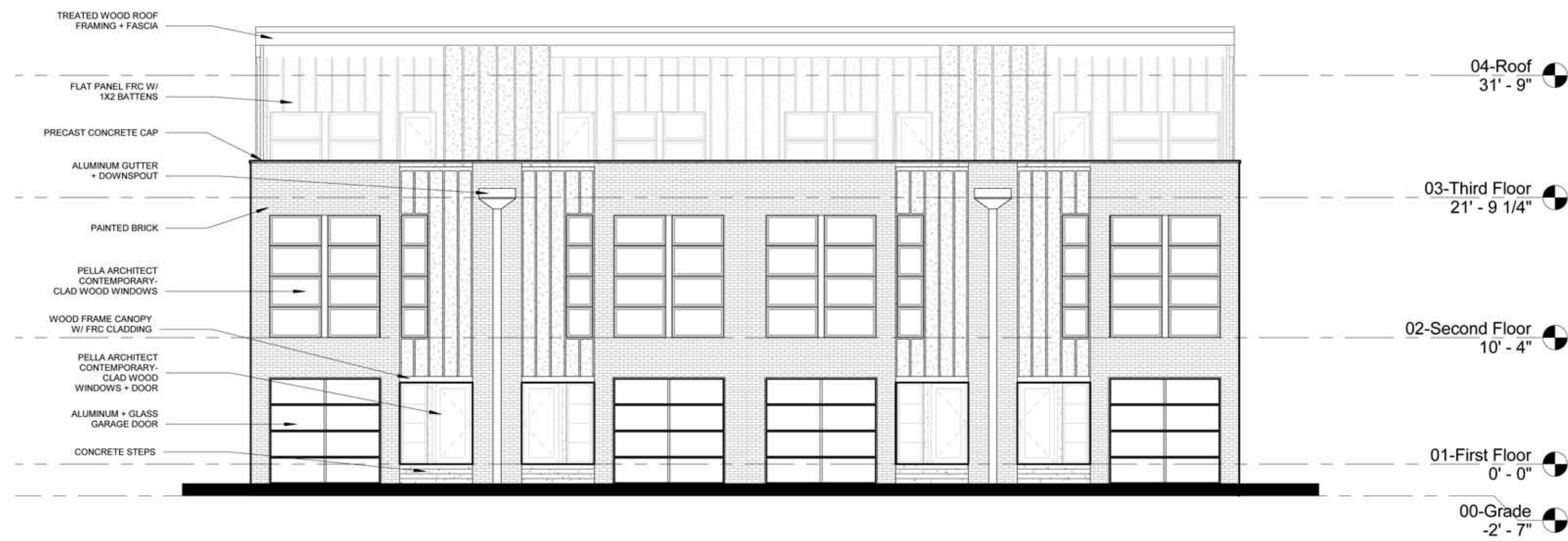
INTERIOR UNIT PARKING COURT ELEVATION (east)
