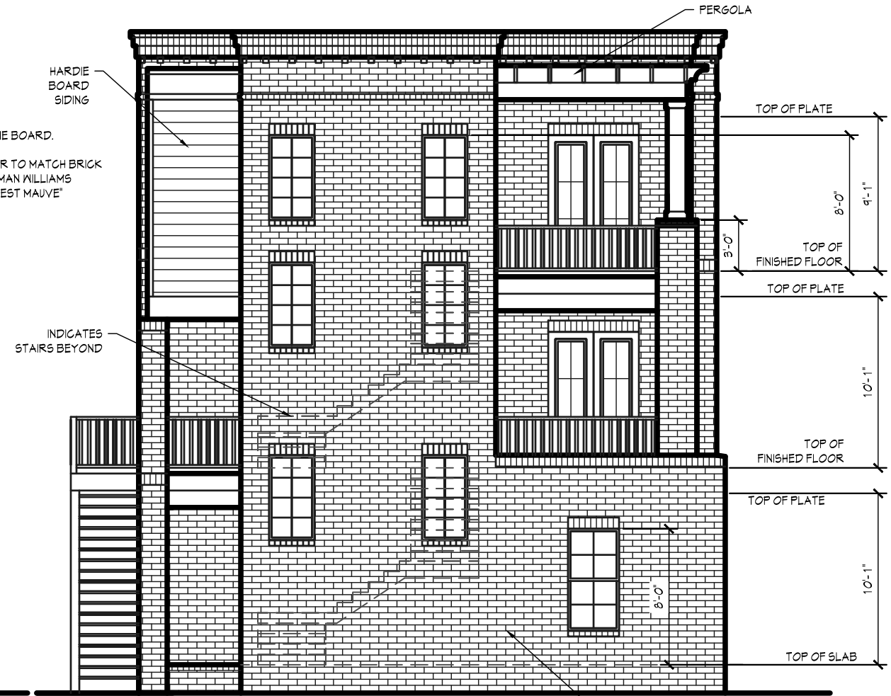
LEFT ELEVATION SCALE: 1/8"=1'-0" APPROVED BRICK SEE OWNER FOR BRICK AND MORTAR COLOR
