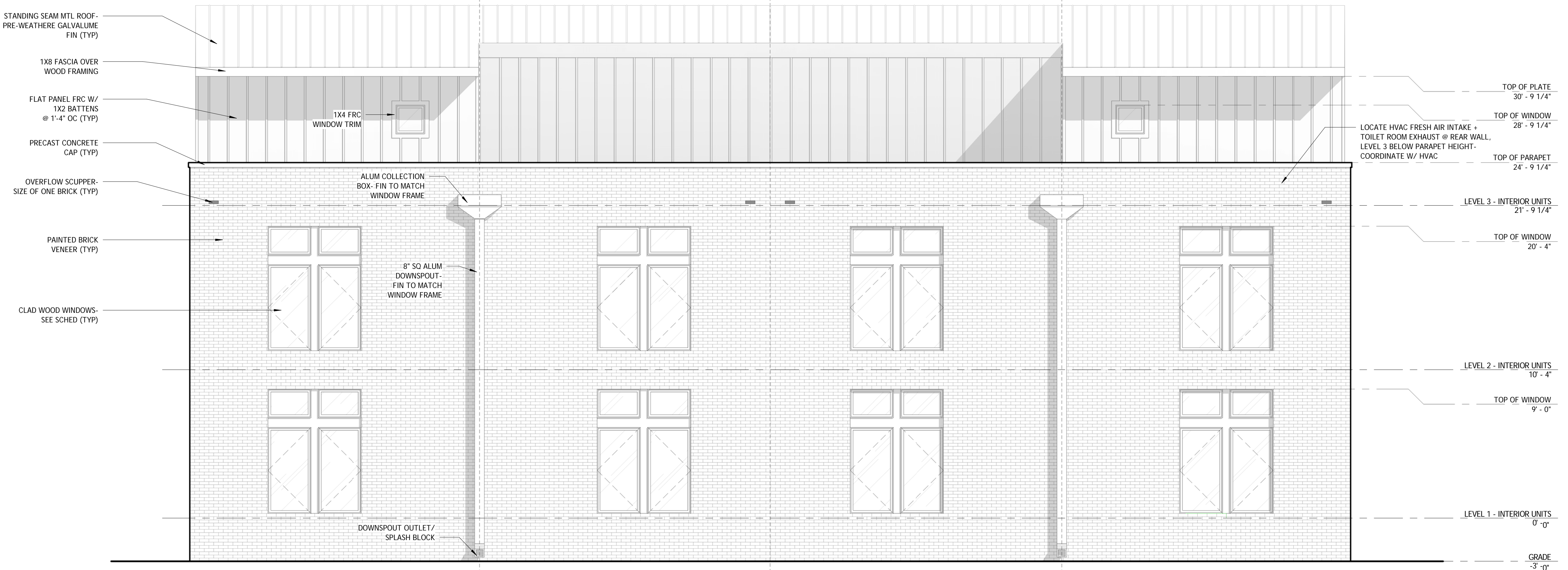
2 INTERIOR UNIT GARDEN ELEVATION - WEST 1/4" = 1'-0"
