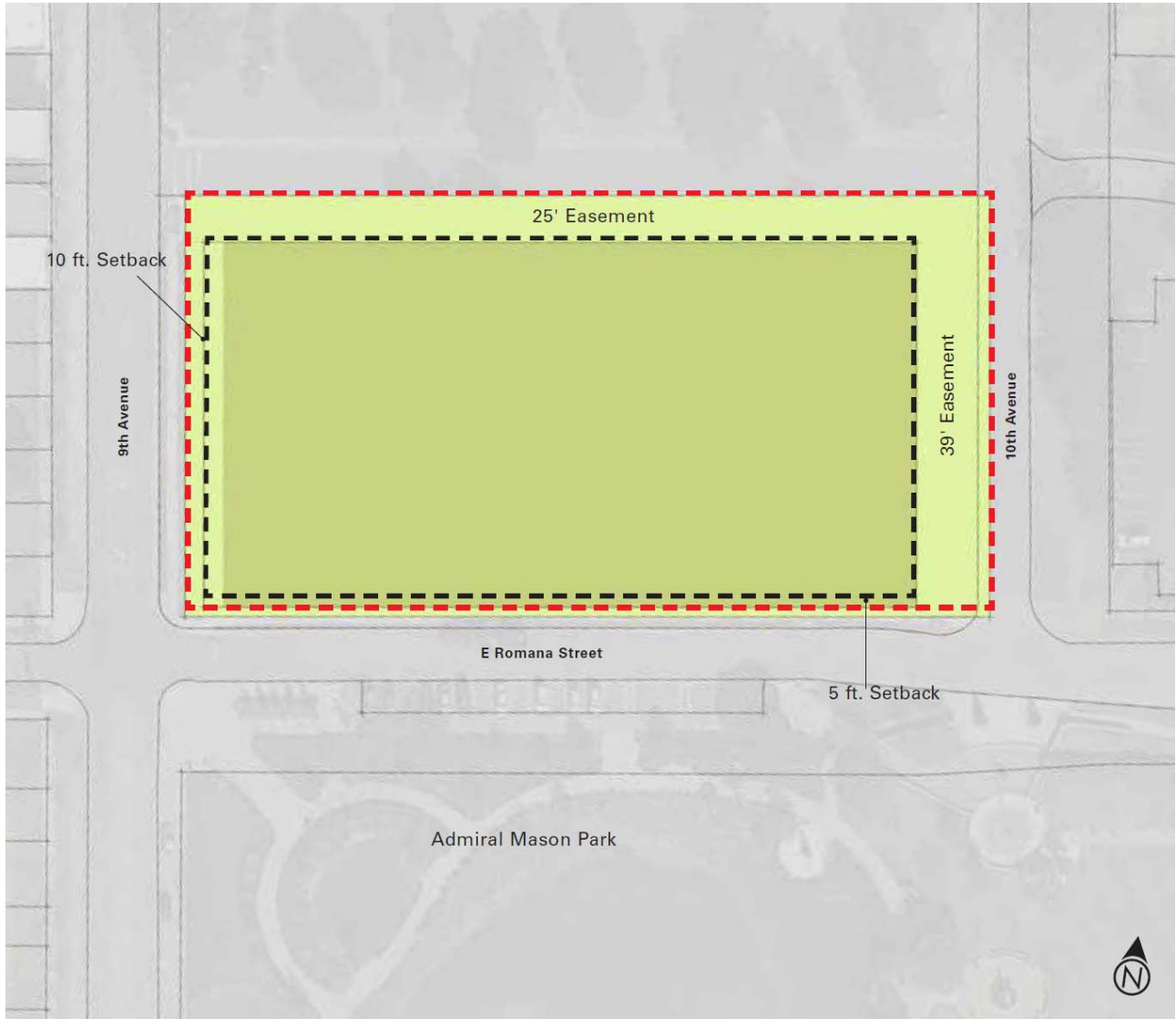
Hawkshaw site setbacks and easements (For illustrative purposes only; reference scaled property survey)
