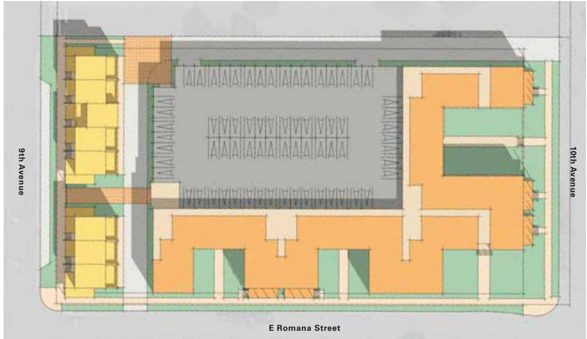
Option 2 — Illustrated ground floor plan showing distributed open space between multi-family buildings
