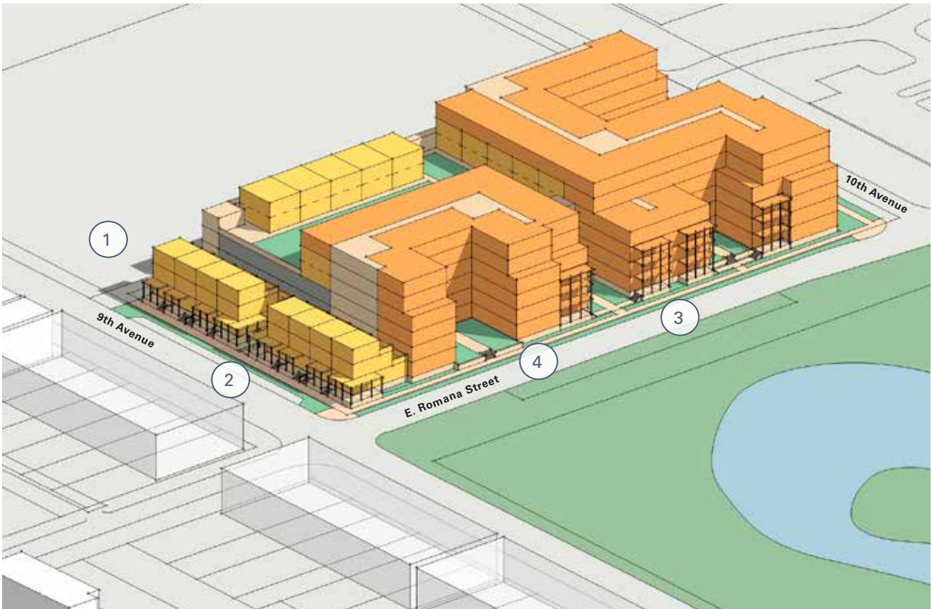
Typical articulation with galleries and porches to achieve Pensacola character and maintain 4 story read for facades along Romana S
