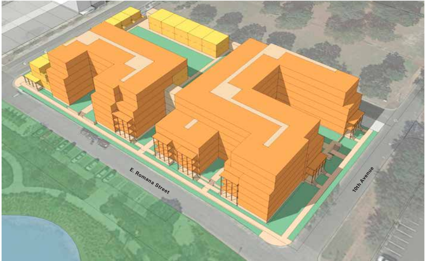
Option 1 — Illustrated view of 6-story massing with galleries and building setbacks along Romana Street. Townhouses are shown facing 9th Avenue and lining the garage courtyard.
