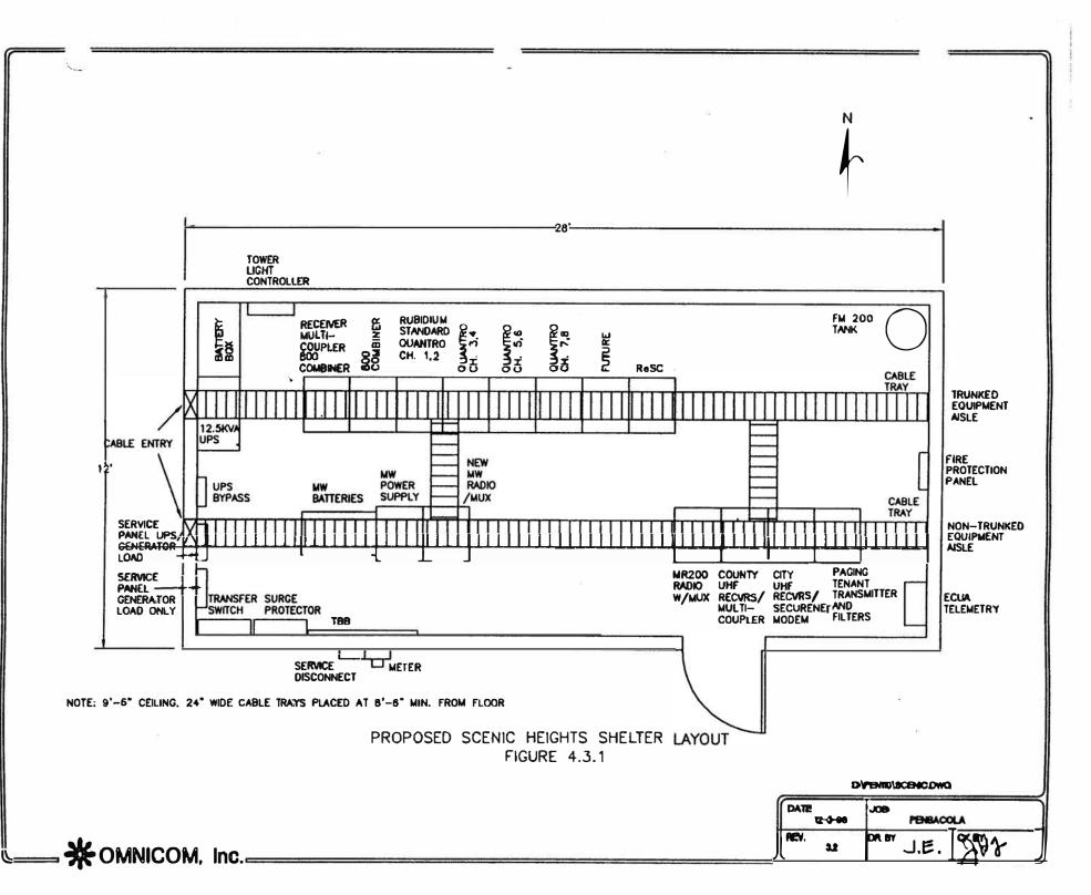
A four-plex grounded receptacle group shall be installed on the outside of each cable tray at typical 20.5 inch intervals corresponding to equipment rack locations. Each duplex receptacle of the four-plex group shall be protected by a separate 20 amp circuit breaker.
