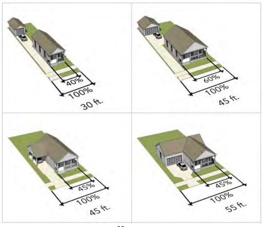
b. The outer edge of driveways shall be placed a maximum of two feet from either side property line. See Illustration 12-2-25.10 for a depiction of driveway placement for single family detached and two-family attached (duplex) buildings on 30' wide lots.
