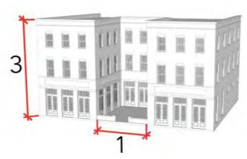
(c) The design and façade treatment of mixed-use buildings shall differentiate commercial from residential uses with distinguishing expression lines (such as cornices, projections, banding, awnings, terraces, etc.), changes in fenestration, façade articulation and/or material changes. See Illustration 12-2-25.5 for depiction of mixed use building differentiation of uses.
