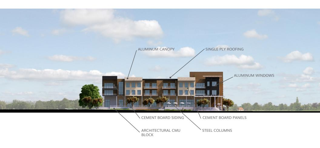
NOTE: NORTH AND EAST ELEVATION MATERIALS WILL BE SIMILAR EX-CEPT METAL ROOFING AND STUCCO FINISHES MAY BE INCLUDED IN THE PALETTE
