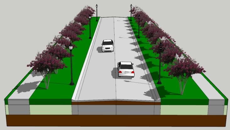
The existing typical section and proposed typical section dimensions are identical. The only additions are sidewalks, street trees, and lighting. No change is proposed for the right-of-way or travel lane widths.
