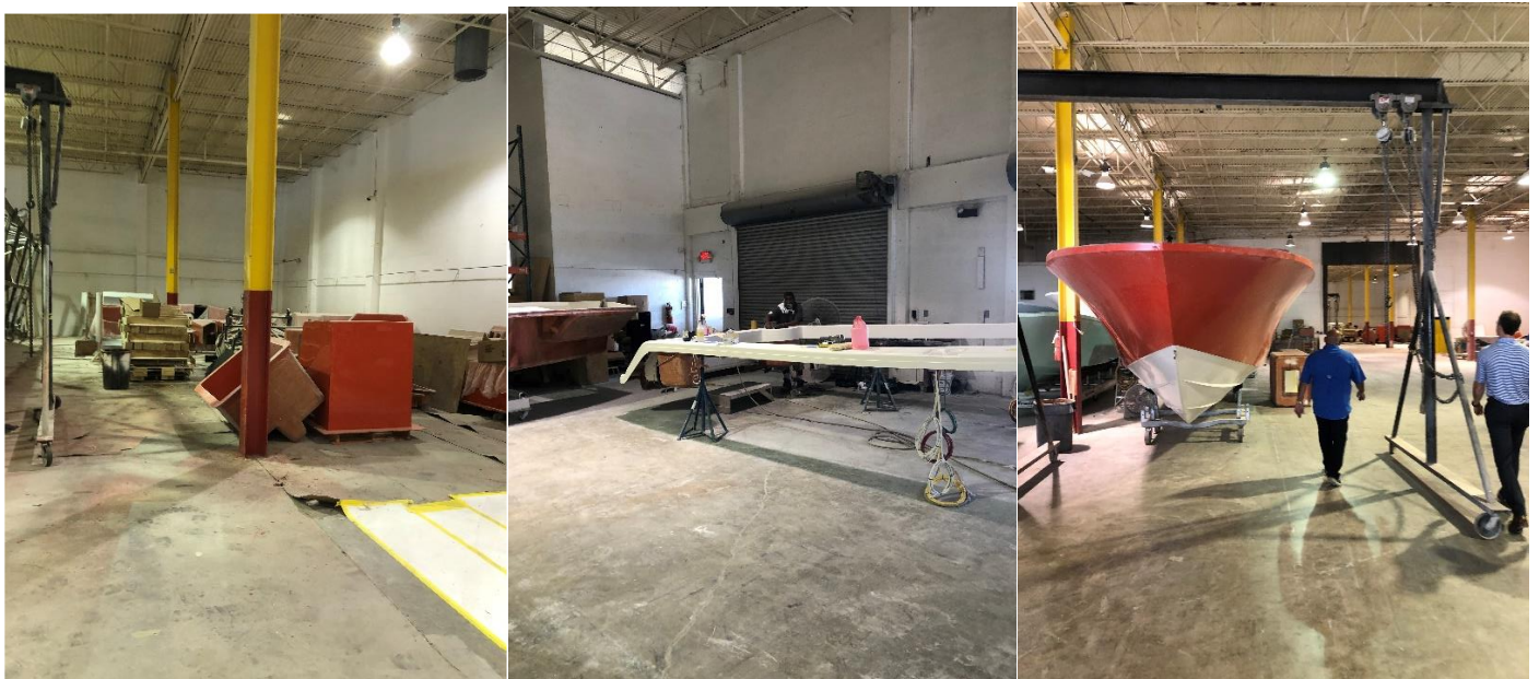
(From left to right) Storage area in hull fabrication room; top of boat railing being finished and prepared for mounting on boat; in the main fab room a finished hull being is prepared for topside center console mounting. Note the clear opacity within the warehouse and the clean shop floor.
