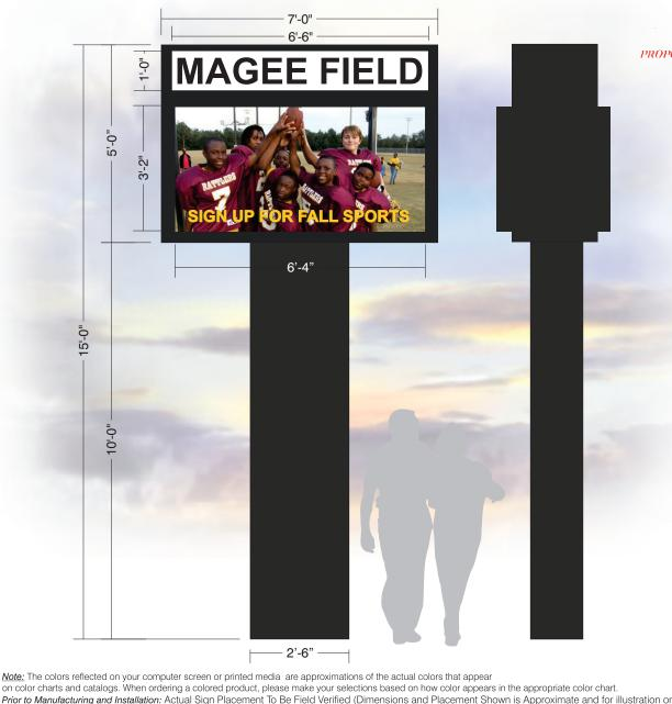
PROPOSED ELEVATION SIZE & PLACEMENT ILLUSTRATION IS APPROXIMATED All Sizes & Exact Placement To be Field Verified Survey Required Shown For illustration / Concept
