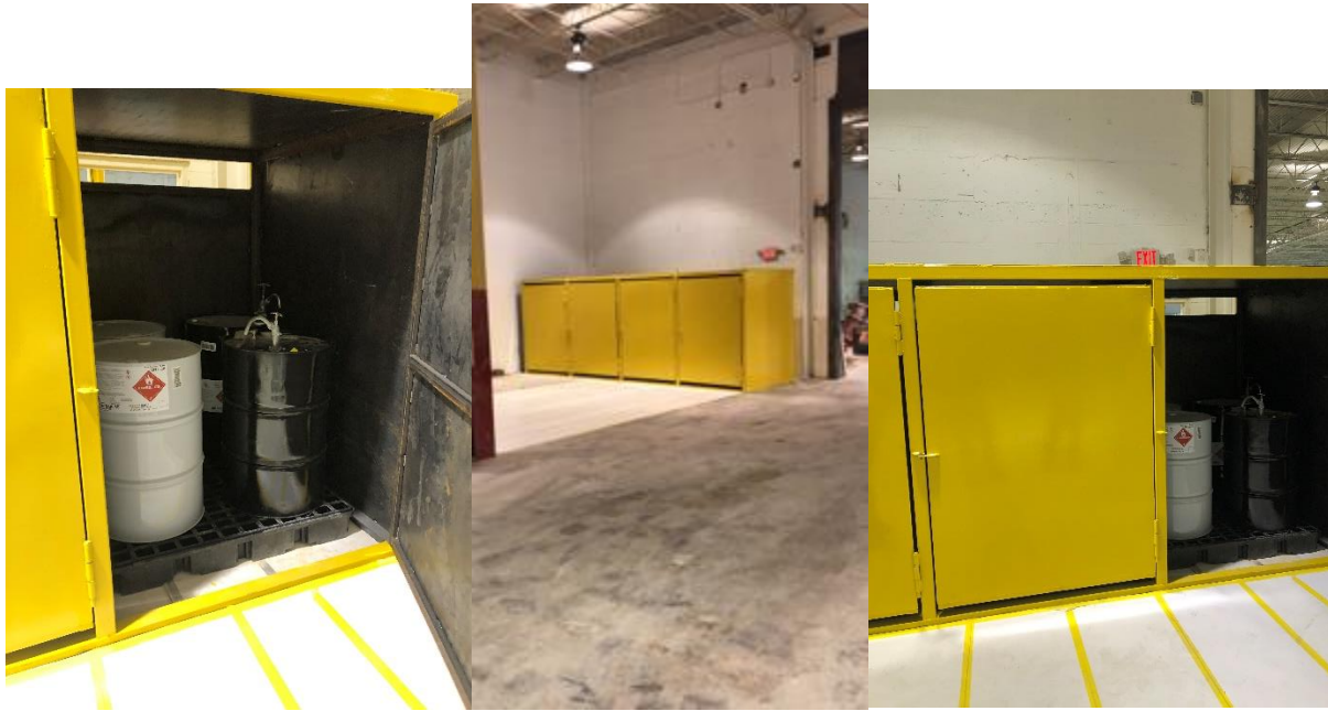
Hazardous materials storage area located in the hull fabrication of the warehouse. Note barrels are stored on elevated pallets.
