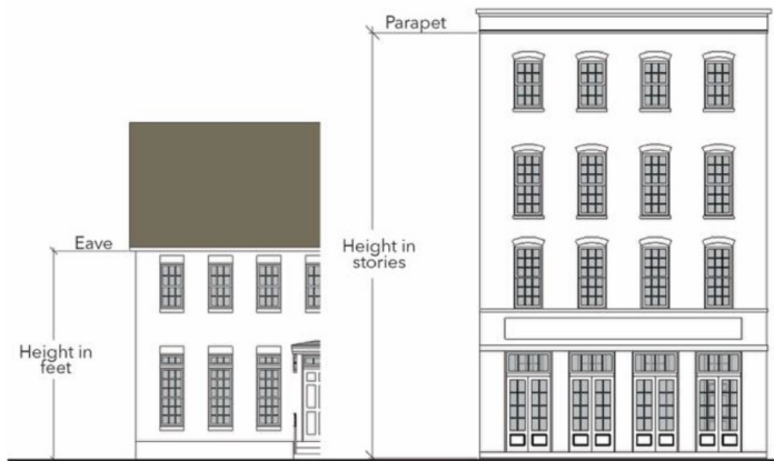
Illustration 12-2-25.1 - Measuring Building Height
