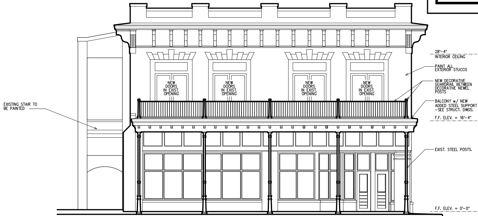
1 A2.1 East Elevation NEW WORK 3/16"=1'-0"
