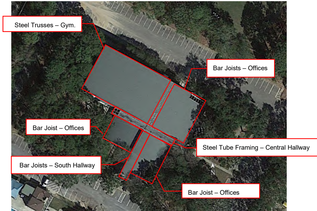
Figure 14: Roof Framing Layout - Vickrey Center
